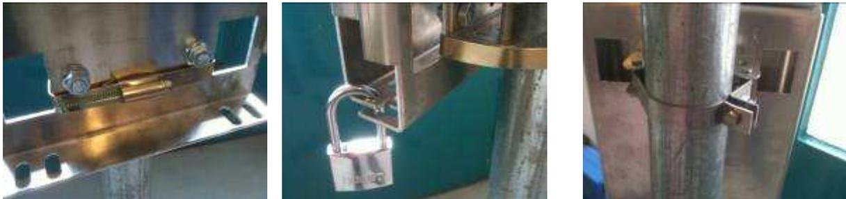
Special plate can be installed on the pole and the speed sign can be mounted and unmounted by a padlock.
